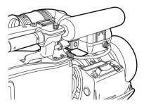
4 Connect the microphone connecting cable to the MIC IN jack.
